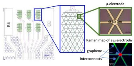
**Figure 2:** Graphene  $\mu$ -electrode arrays
