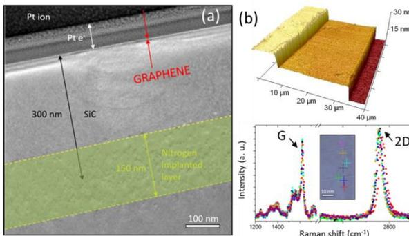
**Figure 1:** (a) Cross-sectional high-resolution transmission electron microscopy micrograph of an ion implanted (nitrogen) SiC substrate covered with an EG layer. The implanted layer has been highlighted in yellow for the sake of clarity; (b) Atomic force microscopy image (top) and Raman measurements collected at several points located on the surface (bottom) of a selected sample showing the relief and the characteristic peaks of EG grown on SiC, respectively.
