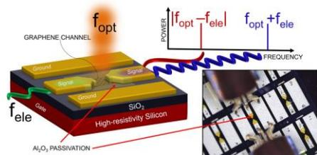
**Figure 1:** Optoelectronic mixer based on CVD graphene
