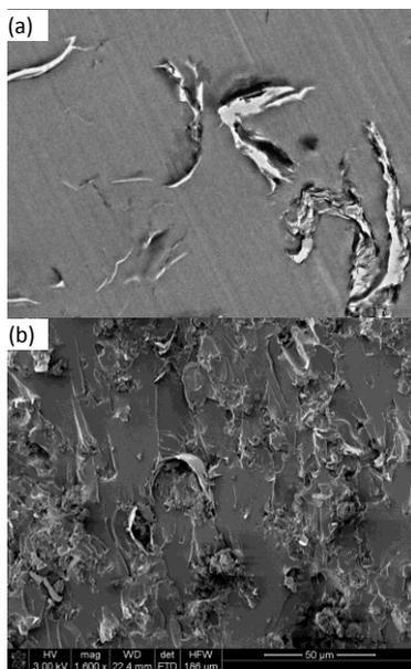
Figure 1: Benzoxazine nanocomposites with 2 wt.% rGO: TEM (a) and FEG-SEM (b) micrographs.
