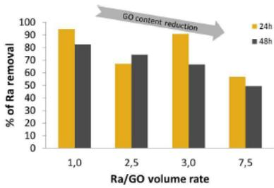
**Figure 1:** Percentage of Ra removal obtained as a function of Ra/GO volume rate and mixing time.
