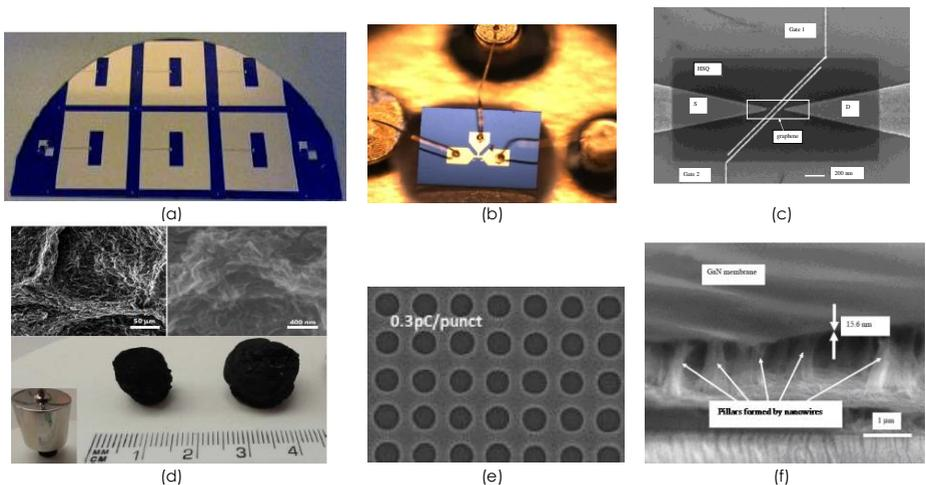
**Figure 1:** Some results: (a) graphene antennas for microwaves in X band (b) graphene FET with 10<sup>4</sup> on/off ratio (c) graphene ballistic FET at room temperature (d) graphene aerogel for pressure sensors (e) nanopatterned graphene (f) GaN membrane artificial synapse.
