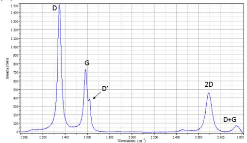
**Figure 1:** (a) SEM image of graphene nanowalls (bar scale of 100nm) (b) Raman spectra of multilayer graphene nanowalls
