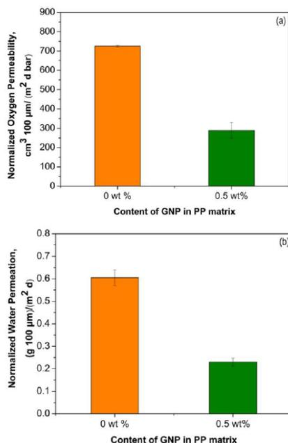
**Figure 1:** Normalized oxygen permeability (a) and normalized water permeation (b) of PP and GNP/PP foils.
