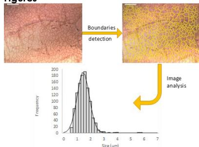
**Figure 1:** Process for grain size characterization. Sample after photocatalytic oxidation with clearly visible grain boundaries (top left), after
